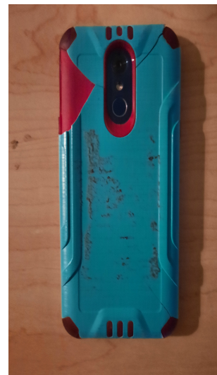
Figure 2. Back The LG Stylo 4 Phone with the Biometric Fingerprint Scanner
